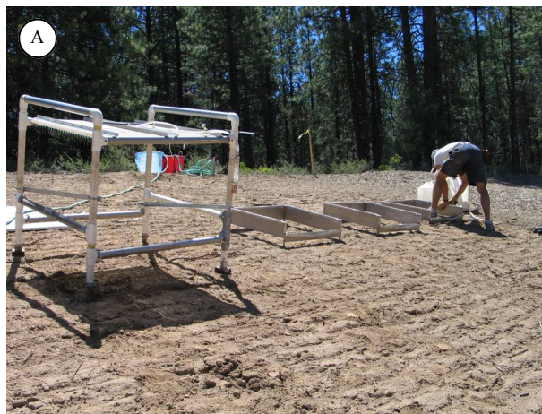
Figure 4. Rainfall simulation was conducted on three plot frames for each treatment. Plot frames are laid out on the soil surface to capture all runoff (A). The rainfall simulator is centered directly over each plot and rainfall is applied. Rainfall is simulated through a series of syringe needles under equal pressure (B). Runoff that occurs within a plot is collected at the bottom of the frame in a plastic bottle (C).
